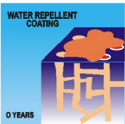
Surface film of film formers No penetration due to micro particle size
