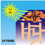
Crack formation due to wind erosion & thermal degradation causing water seepage
